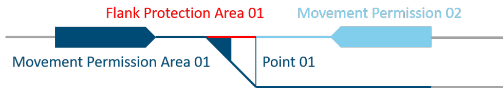
Figure 5: ETCS Vehicle movement is authorised by APS and protected against flank collision
