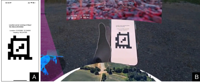
Figure 8: (A) Screenshot of the companion application running on an iPhone. (B) IGUANA MR application scanning the AprilTag displayed on the companion application.
