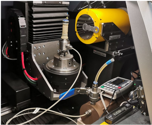
Fig. 12 A sand specimen and a volume-pressure controller inside of the \mu CT chamber
