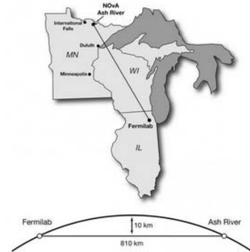
The 500-mile (800 km) subterranean path of the NOvA neutrino beam (Fermilab)
