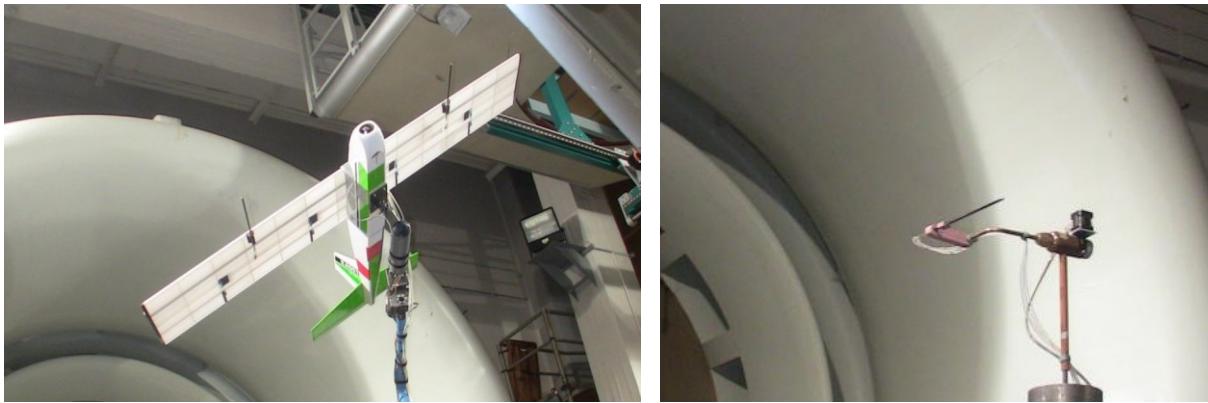
Fig. 3 UAV UrbanCondor (left) and pressure probe (right) mounted in the test section.
