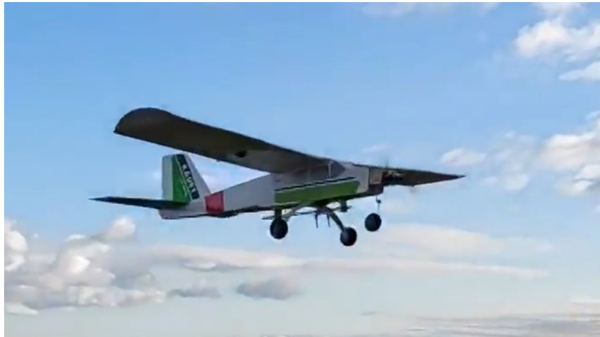
Fig. 1 UAV UrbanCondor carrying a payload mockup during its maiden flight.
