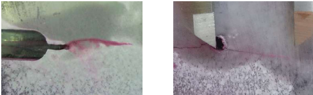
Figure 6. Dye penetrant inspection; left: After the first test phase (specimen “welding 01”); right: after Second test phase (specimen “welding 01”).
