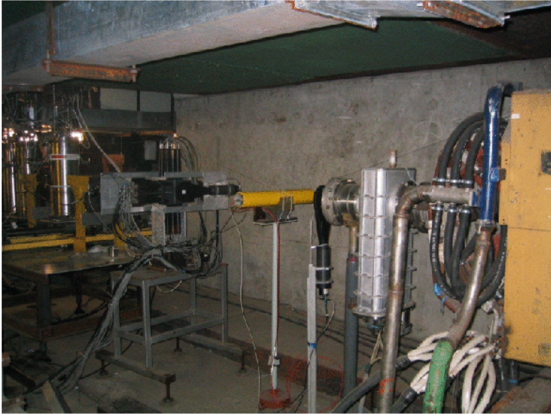
Figure 6.5: Beam area of the Protvino hilumi testbeam. Here the beam direction is from right to left. The devices visible from right to left: secondary emission chamber, scintillation counter S1, ionisation chamber (barrel in the middle of the picture), counter S2, hodoscope and the three cryostats.
