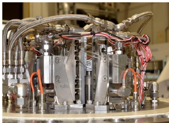
Figure 4: Tribometer assembly periphery (left), friction and wear measurement assemblies (right)
