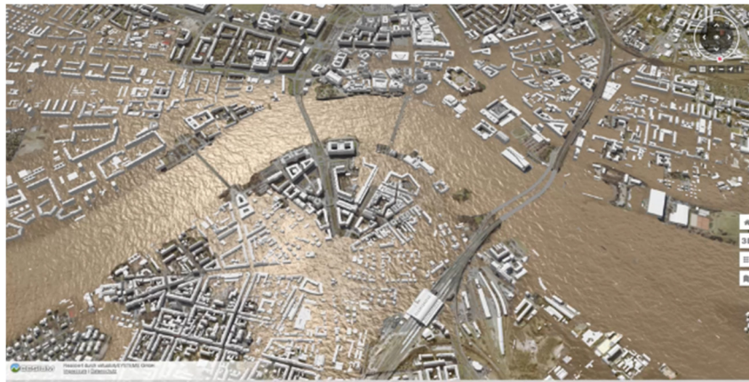
Fig. 2. Example of photorealistic flood scene in web portal (animation based on 2D-simulation results)
