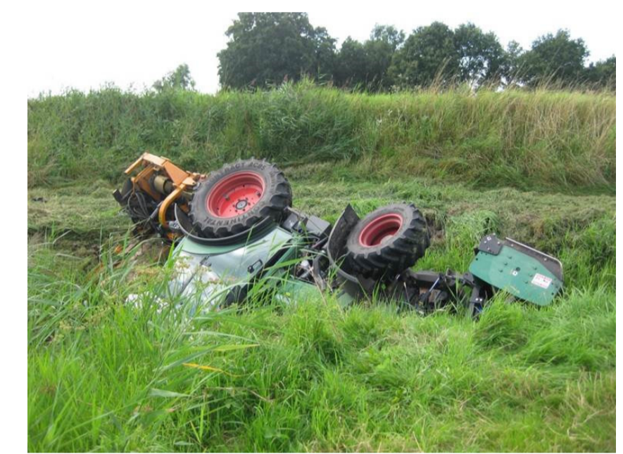
Figure 4 – Accident during river maintenance works due to cavities (Photo: Van der Steen)
