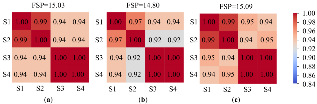
Figure 7. Comparison of the correlation matrices and the frobenius scalar product (FSP). (a) Without sensor anomaly, without structural anomaly; (b) with sensor anomaly in sensor S2, without structural anomaly; (c) without sensor anomaly, with structural anomaly between sensors S2 and S3.
