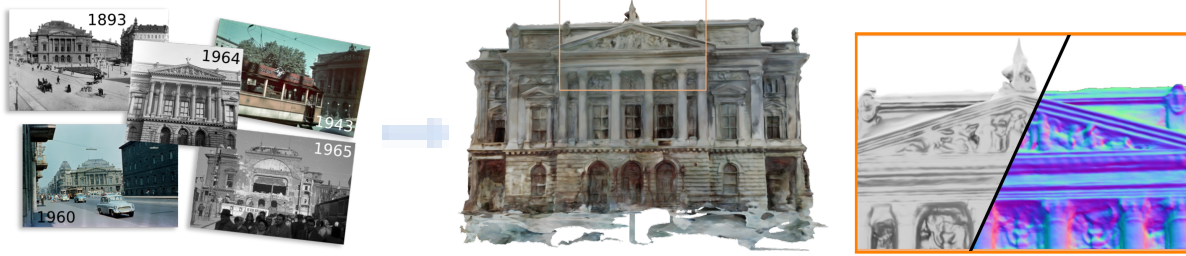
Figure 1. Coloring the Past: Reconstructing high-quality historical buildings from limited data and recovering color appearance from a majority of gray-scale images. The figure shows photographs of the Hungarian National Theater over a long time period (left), reconstructed mesh with color (middle), and shaded mesh + normal map (right).
