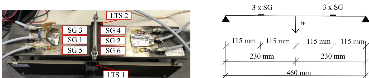
Figure 1: Test setup for the investigation of sensor degradation in strain gauges (SGs) with the use of a displacement-controlled load using laser triangulation sensor (LTS); left: realized test setup, right: idealized static system.
