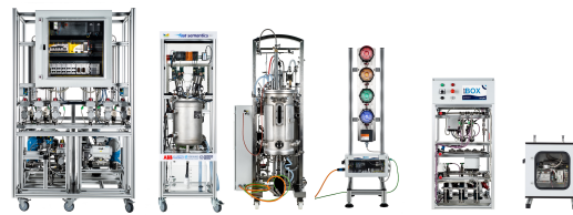
Fig. 2. Examples of P2O-Lab’s Modular PEAs (left to right): Mixing PEA, Parallel-Dosing PEA, Bioreactor PEA, Signal-Light PEA, Media-Supply PEA, Control PEA
