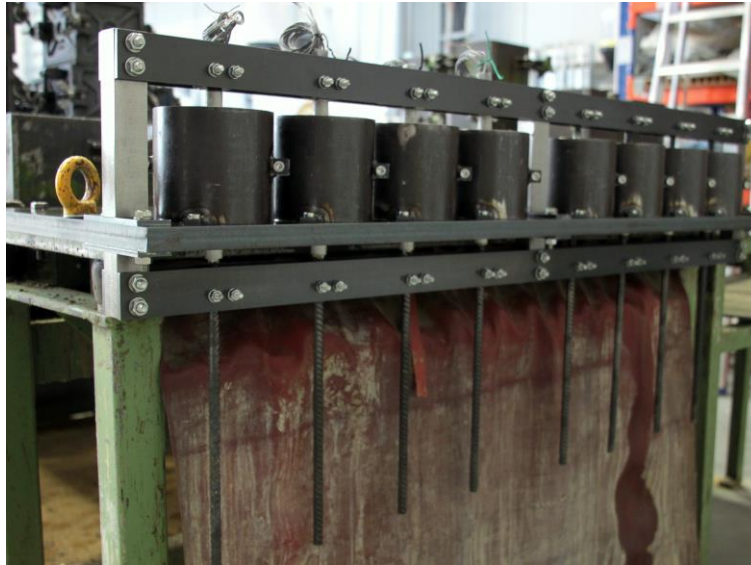
Figure 3-9: First type of formwork for casting cylindrical specimens.
