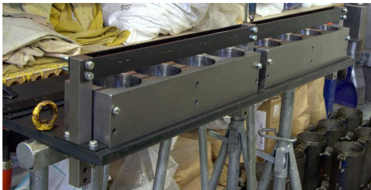
Figure 3-10: Second type of formwork for casting cylindrical specimens.
