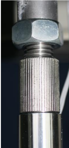
Figure 3-22: a) steel rebar with coupling, b) bolt connecting the rebar to the transfer bar.
