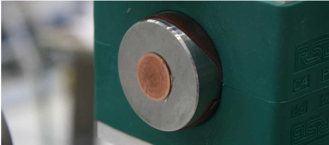
Figure 3-30: Pulse shaper attached to IB1 with a green clamp for stopping the IB1 after 100 mm.
