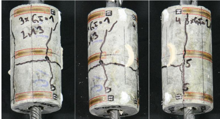
Figure 2-8: Example of splitting failure.
