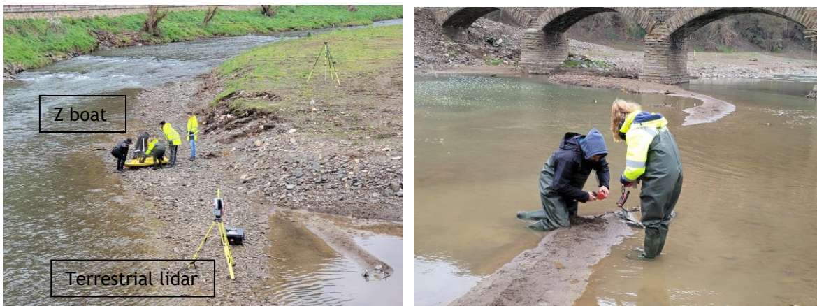
Figure 16. Left) Deployment of Z-boat for bathymetric measurements in the Ahr river in just upstream of the town entrance of Altenahr. Right) Sediment sampling in the same location.
