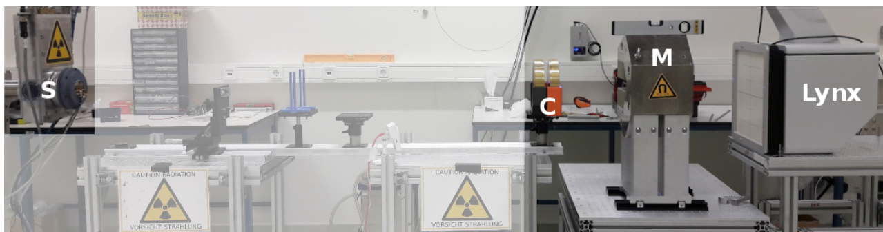
Figure 5.3: The two cylindrical brass collimators (C) are positioned at 168 cm from the beam snout (S). The magnet (M) to Snout distance amounts 202 cm. For the transmission experiment additionally the Lynx detector is placed 26 cm behind the magnet.
