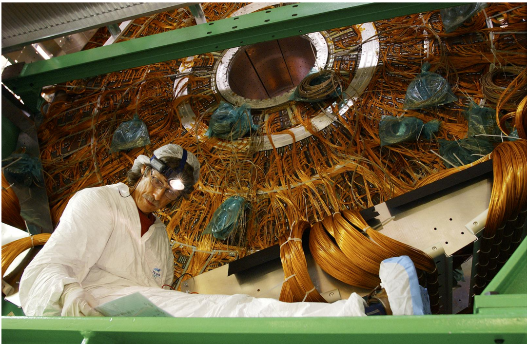
Figure 1.2: A technician for the ATLAS collaboration, Michel Mathieu, cabling the electromagnetic end-cap [9].
