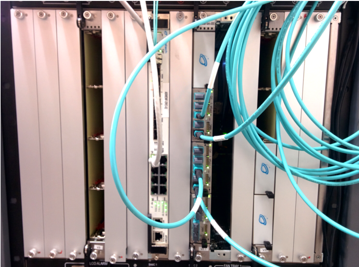
Figure 4.7: A test setup of the prototypes of the LATOME hardware at EMF at CERN
