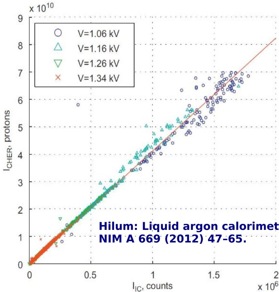
**Hilum: Liquid argon calorimeter performance at high rates**
