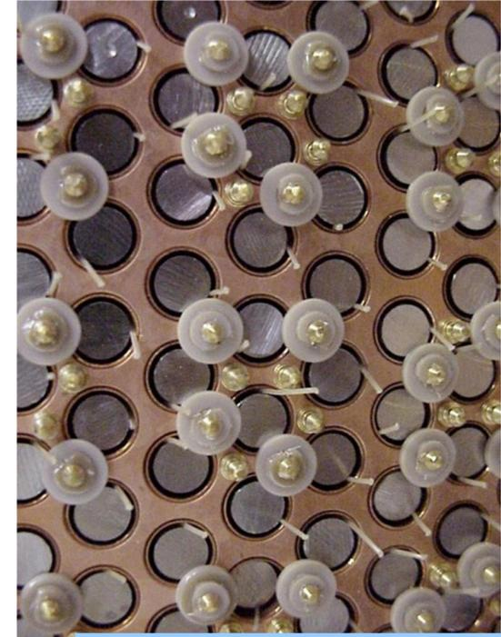
**Electrode Rods & Absorber Matrix**
