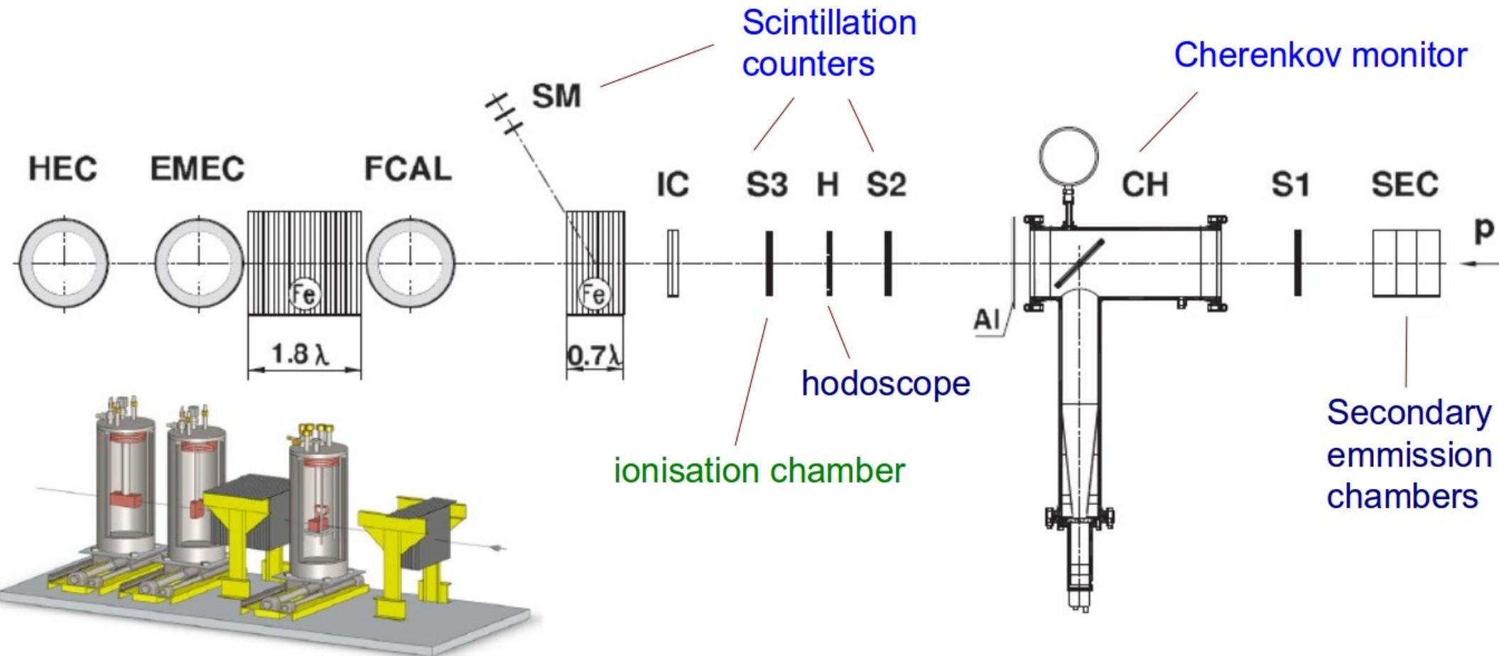
Test beam setup and absorber thickness was optimized in MC
