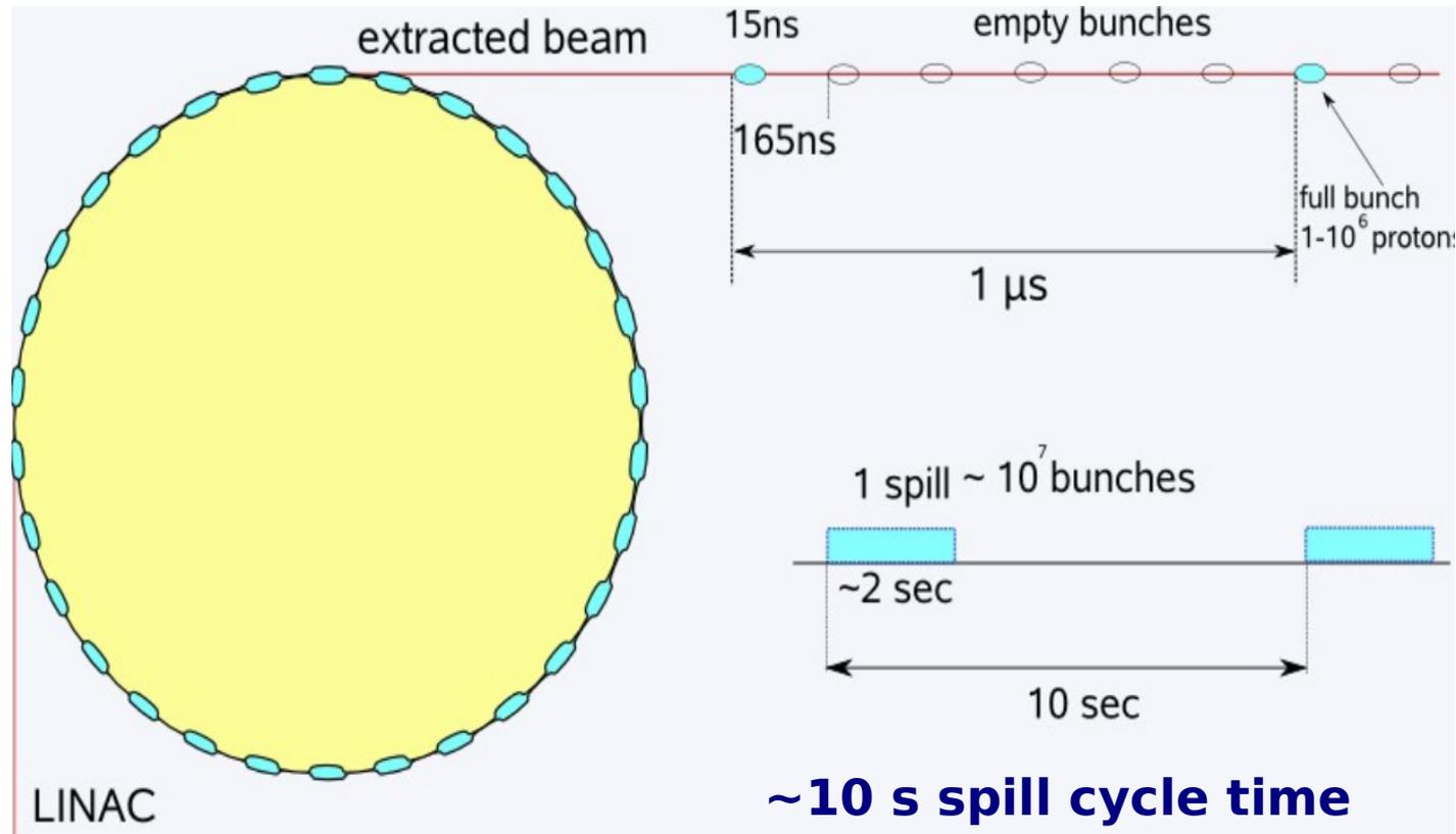
**Intensity range:  $10^6$  -  $\sim 3 \times 10^{11}$  p/spill**
