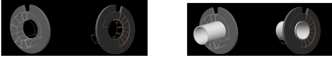
Figure 3.3: Construction of a range modulation wheel. The left plot shows a range modulation wheel without a shell and a hub to visualize the 10 lexan steps for range modulation in the upper section (left, white) and the corresponding lead steps at the bottom section (right, brown) for scattering compensation. The right plot includes an aluminum shell and an aluminum hub.
