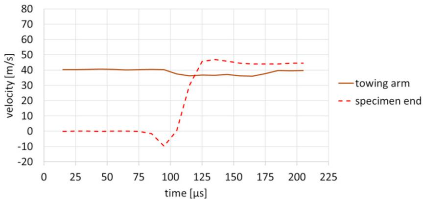
Fig. 4. Velocity vs. time curve of the towing arm and the accelerated specimen end at a test speed of 40 m/s
