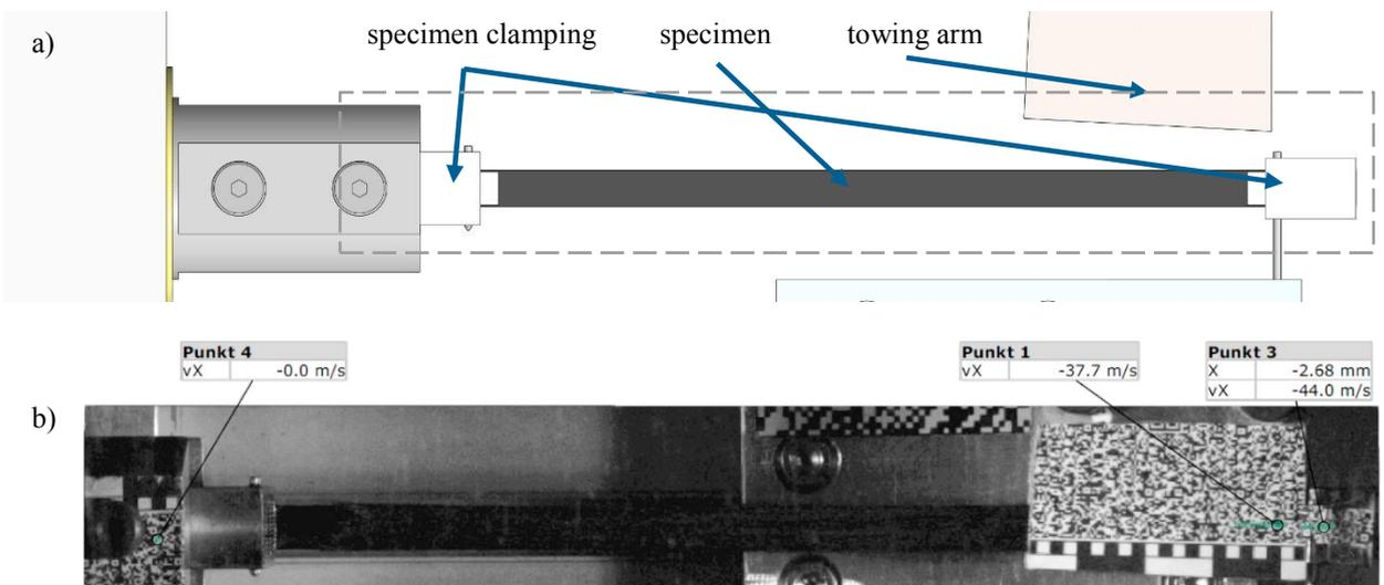
Fig. 2. (a) principle set-up of the specimen holder with marking of the screenshot area; (b) Screenshot of DIC-analysis at the moment of impact
