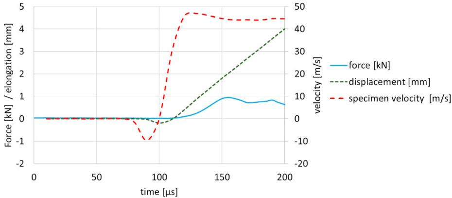
Fig. 3. Response of the force signal, the distance and the speed of the accelerated specimen end at a test speed of 40 m/s
