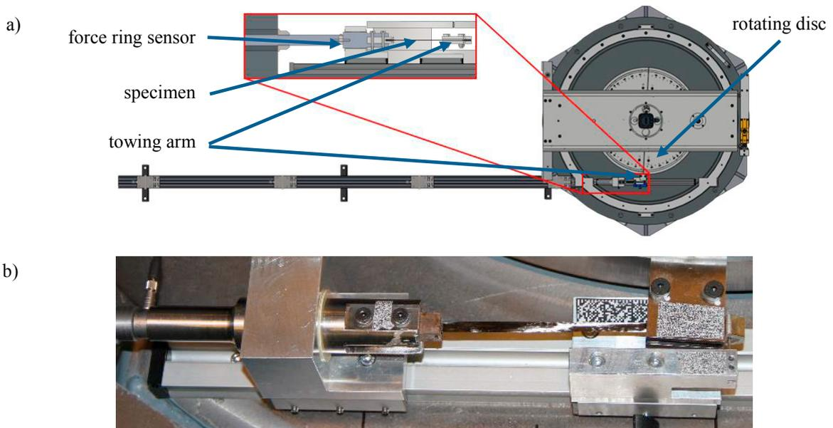
Fig. 1. (a) Test stand with detailed illustration of specimen clamping and force recording; (b) Photo of a clamped specimen with visible DIC markings.
