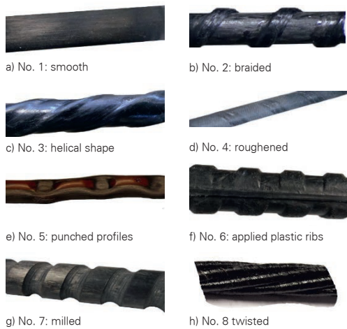
Figure 1: Used carbon rebars | graphic: Alexander Schumann
