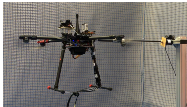
Figure 4 Multicopter with rod-shaped manipulator in contact with the sensor surface.
